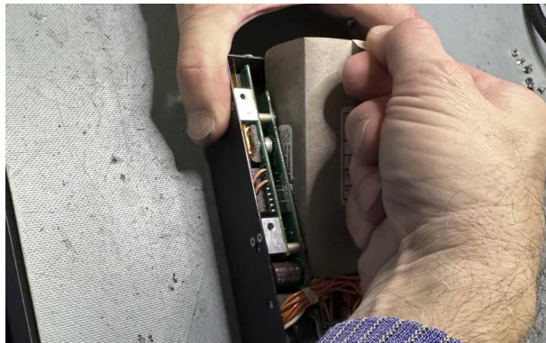
Figure 3: Removing the Battery Pack – Lift by the Tab
