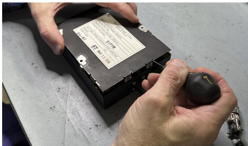
Figure 2: Removing the Lid – Prying it Off
