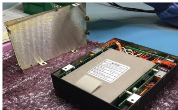
Figure 5: Reinstalling the Lid – Note the 4 Mounting Block Holes and the 7 Perimeter Holes
