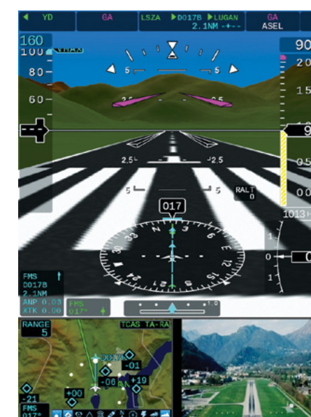
PFD with 360° HSI, Left Inset with Map, SVS, and Traffic, Right Inset with Video
